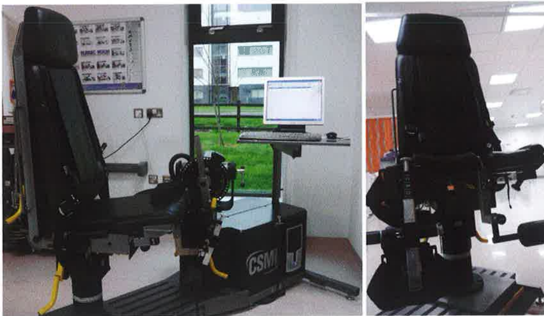
Figure 15: The Cybex isokinetic dynamometry machine with an anti-shear device
